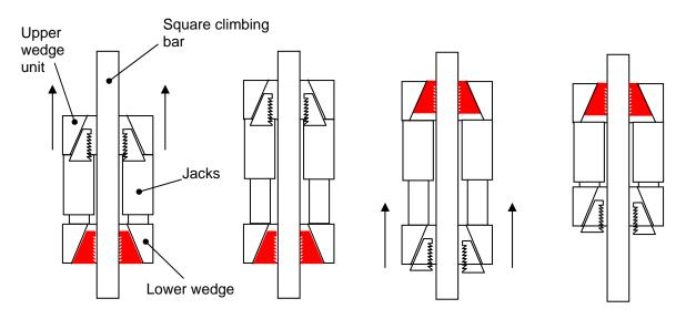
Stage 1 Load held in lower wedge unit Jacks extend to raise upper wedge unit
