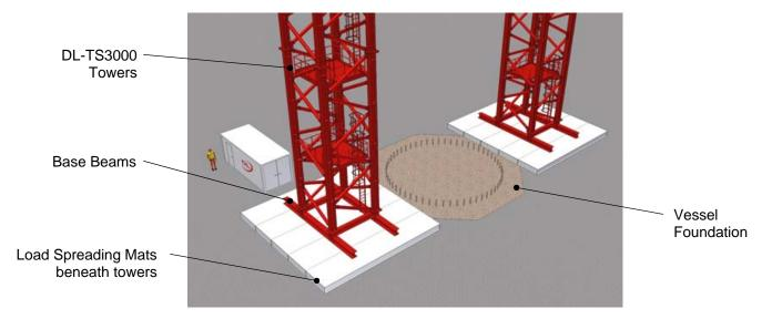
For towers in the freestanding configuration, due to the magnitude of the overturning moments, it is likely that base outriggers with ballasted outrigger trays would be required. This option has the advantage that it does not require any significant civil engineering works. However, it does need sufficient space around the towers for the outrigger trays and reasonable ground conditions under the load spreading mats and outrigger trays.
