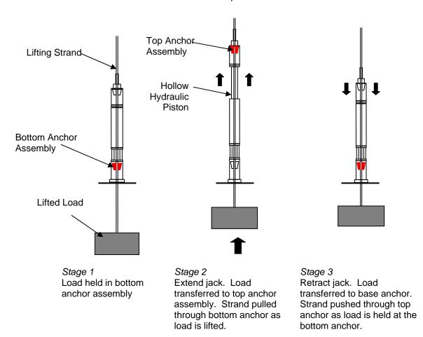
Strand jacks are available in a wide variety of capacities varying from 15 tonnes to 1022 tonnes. Each lifting strand consists of 7 individual wires formed into a single strand approximately 18mm diameter. The minimum-breaking load of each strand is 38 tonnes. Each strand has a working capacity of 15 tonnes, thereby providing a 2.5 factor of safety. Jacks of capacities greater than 15 tonnes, use a series of these strands arranged in a group to achieve the required capacity.
