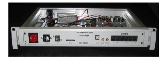
2 independent controllers, one for ECAL TOP, one for ECAL BOTTOM. Clock is propagated from the first to the second for syncronization (feature already tested)
