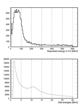
94k events out of 511 from run 1371 Top: deposited energy in CU per event Expected 90 MeV/ $\cos(30^\circ) = 104$  MeV but we have < 100 MeV. Bottom: deposited energy per Xtal per event Expected 11.2 MeV/ $\cos(30^\circ) = 13$  MeV but we have 11 MeV
