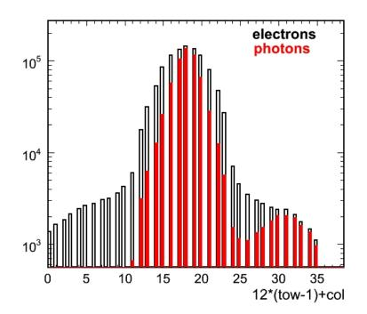
Column hits in CAL as beam check, reproduces nicely the TKR profile.
