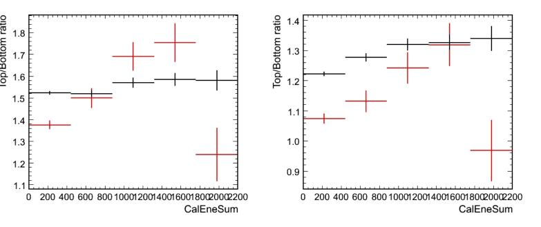
Upward trend, fractional energy deposit in CAL becomes less dependent on vertex height when the energy increases. MC errors large but slight disagreement with data.
