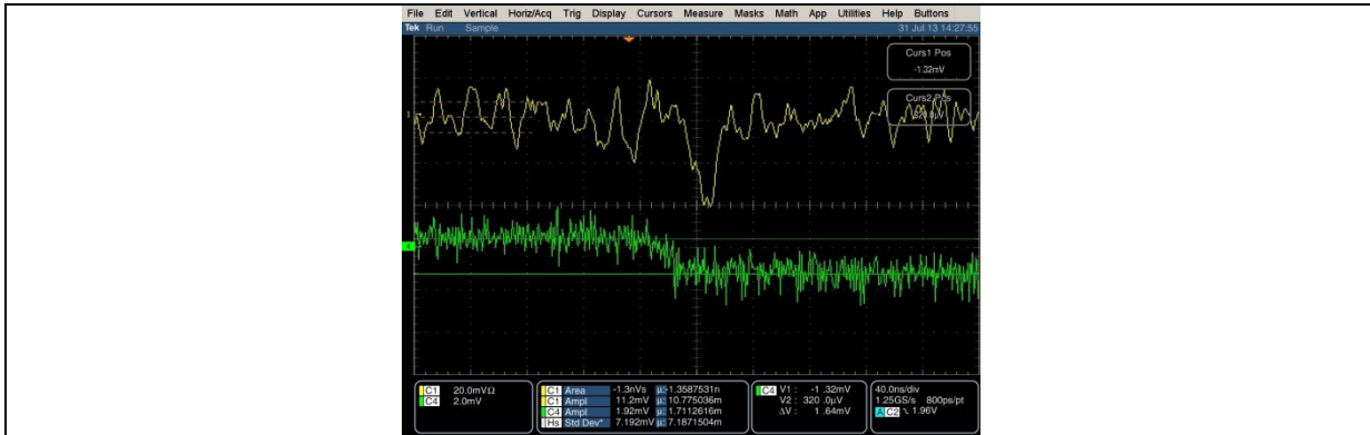
Figure 9: Output signal for Q_{in} = 7.7\text{fC} ( V_{in} = 1.64\text{mV} and 4.7\text{pF} ). The output signal is about 40mV.
