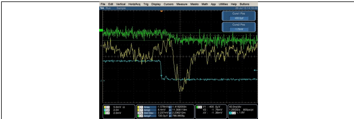
Figure 5: output signal (yellow trace) of the preamplifier N318 and for 6fC as input charge. Without input capacitance.
