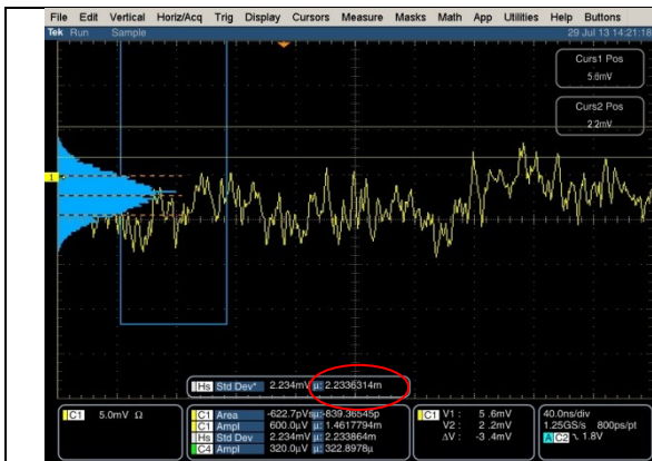
Figure 6a: output noise of the preamplifier N318 without input capacitance. The standard deviation is 2.2mV-RMS.
