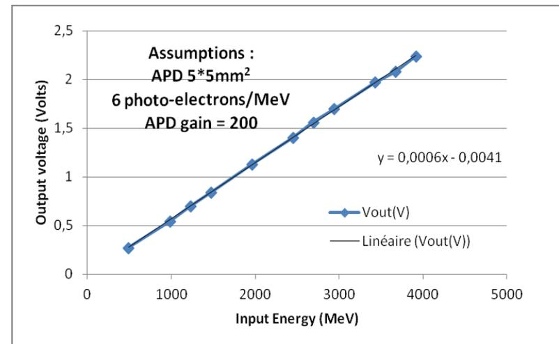
Gain = **3V/pC** (Pulse Width = 20ns) or **0.6mV/MeV** (6 photo-electrons/MeV and APD gain = 200) or **2333 pC/pC** (=1.4nC/0.6pC)
