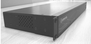
Installed L bracket:
