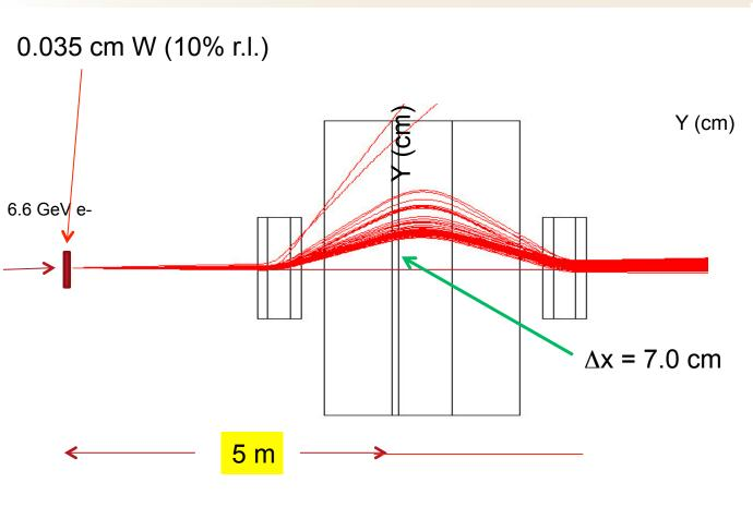
Expect maximum of 8×10<sup>5</sup> electrons/ strip / 40usec Spot size is ~0.32cm width No time evolution – static for 40usec for this example (?)
