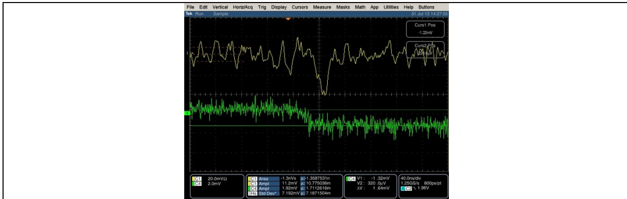
Figure 9: minimum estimated output signal for Q_{in} = 7.7\text{fC} ( V_{in} = 1.64\text{mV} and 4.7\text{pF} ).
