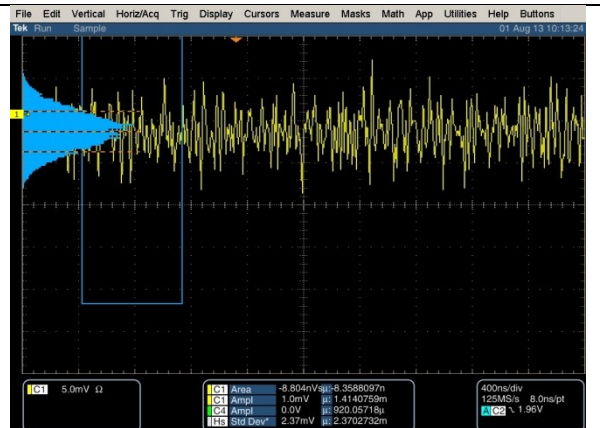
Figure 12b: output noise of the modified FT22 preamplifier with 270pF as input capacitance. The output noise is 2.4mV-RMS.
