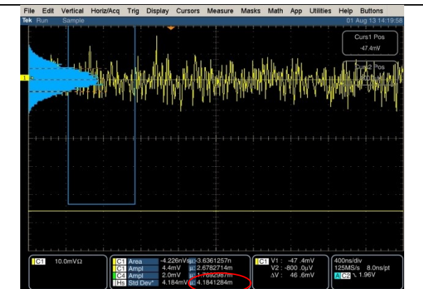
Figure 6b: output noise of the preamplifier N318 with 82pF input capacitance. The standard deviation is 4.2mV-RMS.
