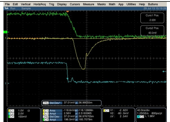
Figure 3b: saturated output signal (yellow) of the N318 preamplifier and for 0.85pC input charge.
