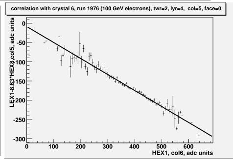
When 100 GeV electron beam hits crystal 6 nonlinearity curve for crystal 5 becomes very different from charge injection
