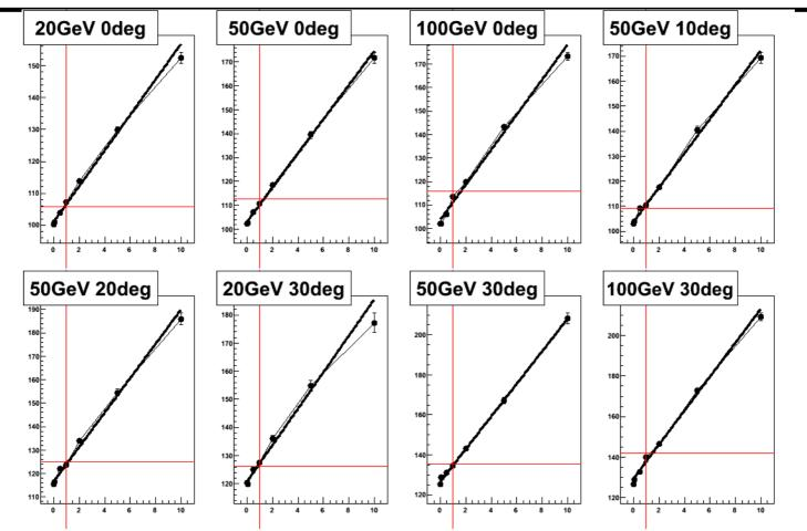
Mean TkrTotalHits as function of pressure (MC black). Horizontal red line gives mean value for data. Vertical red line = 1 bar.
