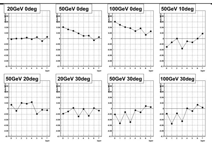
~>O at O deg, ~<O at 30 deg : incompatible with extra XO along the beamline + extra XO in the CU (which would be sensitive to theta)
