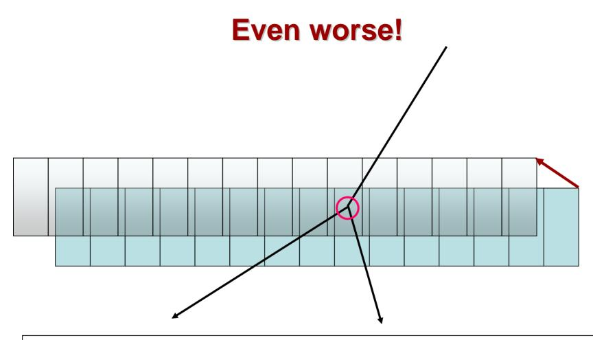
When the offset plane overlaps the ideal one, I try to keep the interaction point at the same place (same space coordinates), which means that the height in the silicon changes, which means that the energy deposit changes.
