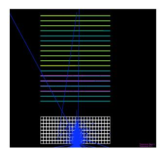
Photons (mostly in E range 0.5-5 MeV) produce electrons in the W and Si planes (Photoelectric or Compton) which can deposit energy in the Si planes (also W planes, of course...)
