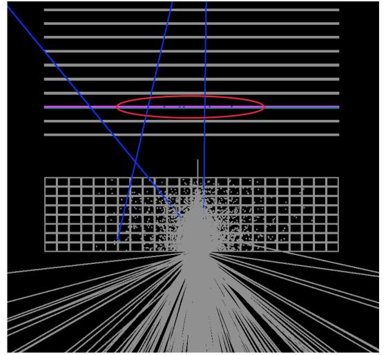
The 3 electrons exiting the calorimeter ("backwards") have large angles and do not go much over the tracker
