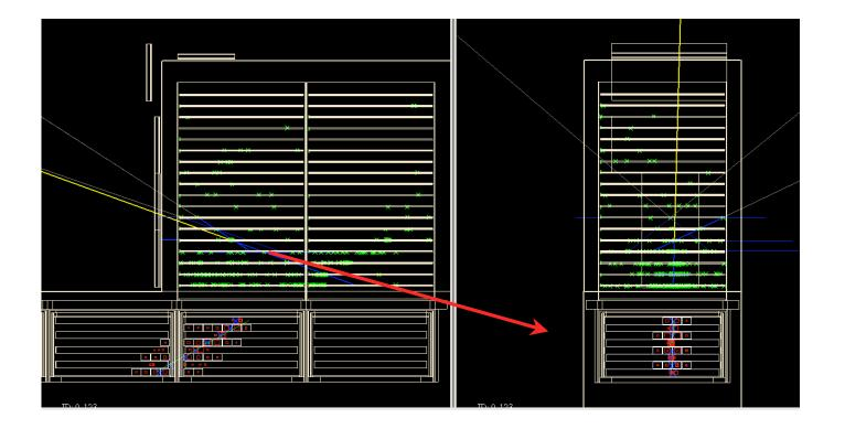
WRONG (random) incoming angle and impact point calculation "Recognized Track 1" is missing the calorimeter 2
