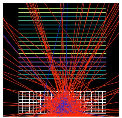
Backsplash can be quantified by computing the energy deposited in the Si and W planes.
