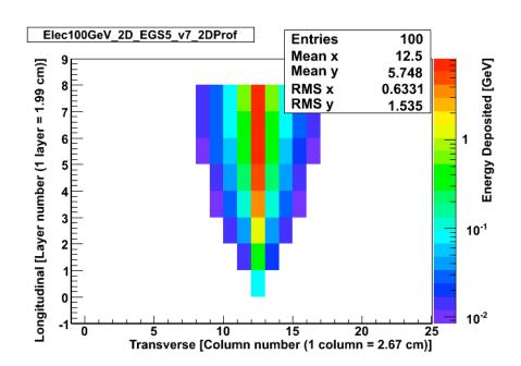
62% of the energy leaks out the calorimeter
