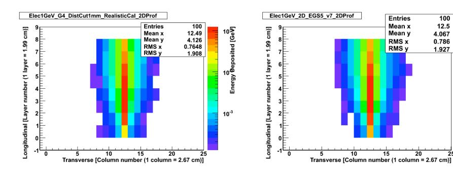
21% of the energy leaks out the calorimeter
