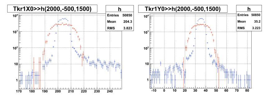
Beam impact point is at the RIGHT position, but MC beam is about 2.5 wider
