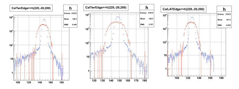
Difference in variables quantifying the distance of the location of energy deposition with respect to the tower edge. This is due to the beam profile differences
