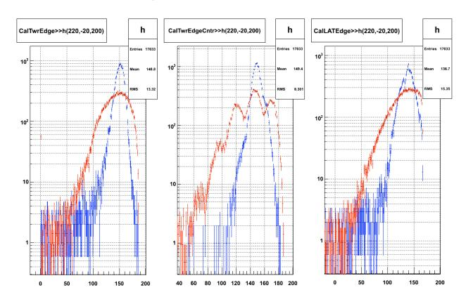
Difference in variables quantifying the distance of the location of energy deposition with respect to the tower edge. This is due to the beam profile differences
