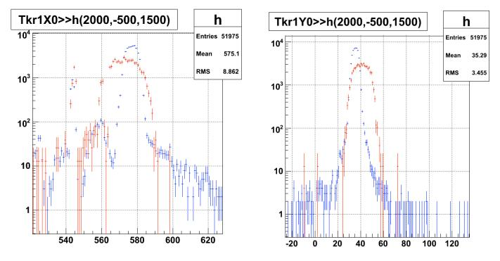
Beam impact point is shifted by ~5 mm, and MC beam is about ~2 wider
