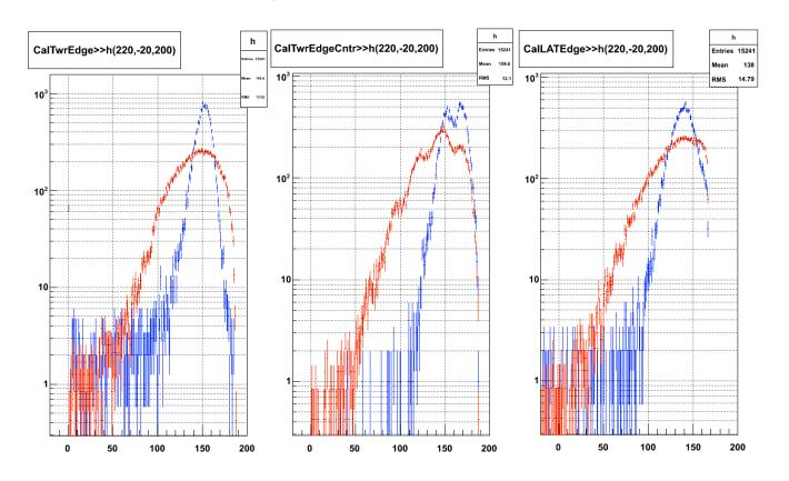
Difference in variables quantifying the distance of the location of energy deposition with respect to the tower edge. This is due to the beam profile differences
