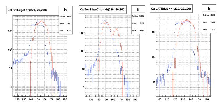
Small shift in variables quantifying the distance of the location of energy deposition with respect to the tower edge. Note that this time the beam profile is correct. This shift is produced by the difference in incoming angle.
