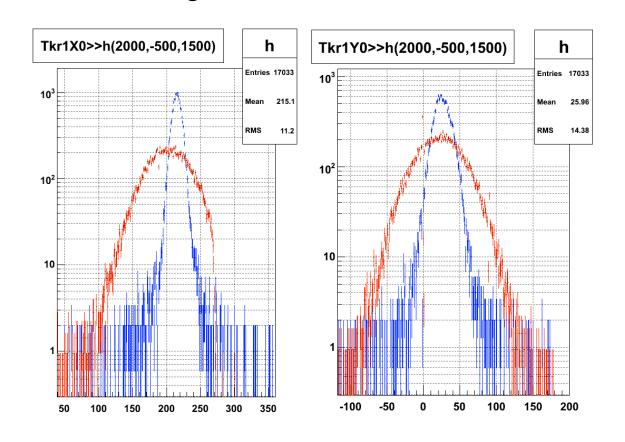
Beam impact point is shifted by ~5-10 mm, and MC beam is about ~2 wider
