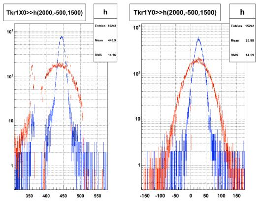
Beam impact point is shifted by ~5-10 mm, and MC beam is about ~2-3 wider
