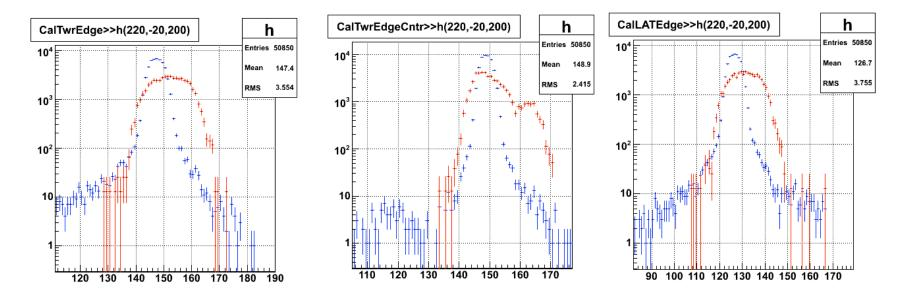
Difference in variables quantifying the distance of the location of energy deposition with respect to the tower edge. This is due to the beam profile differences: beam width and incidence angle
