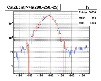
Vertical location of center of gravity is slightly different. This is NOT due to beam profile differences. Perhaps due to differences GEANT 3- GEANT 4
