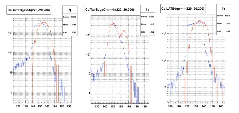
Small shift in variables quantifying the distance of the location of energy deposition with respect to the tower edge. Note that this time the beam profile is correct. This shift is produced by the difference in incoming angle.
