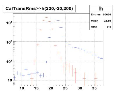
Vertical location of center of gravity is slightly different. This is NOT due to beam profile differences. Perhaps due to differences GEANT 3- GEANT 4 Transverse dimension per single shower is larger in Data.
