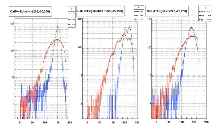
Difference in variables quantifying the distance of the location of energy deposition with respect to the tower edge. This is due to the beam profile differences
