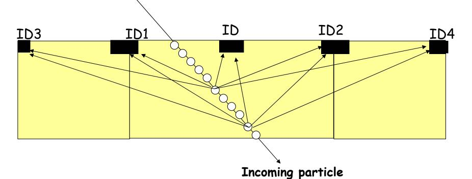
We added the induced charge from each cluster over the strip ID, and so on over the strips ID1, ID2, ID3, ID4 etc.
