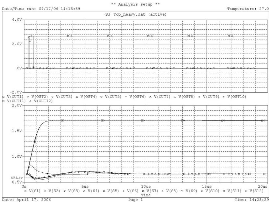
**Figure 4. The comparator response (upper plot) and shaper response (lower plot) to an oxygen ion passing through channel 12.**
