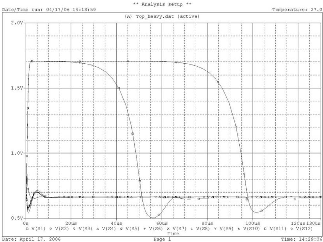
**Figure 3. The shaper response to an oxygen ion passing through channel 12.**
