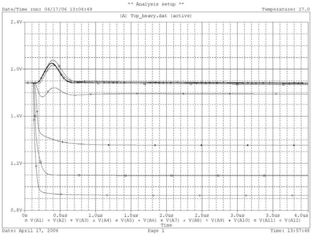
**Figure 6. The amplifier outputs for an iron ion at normal incidence on strip 12.**
