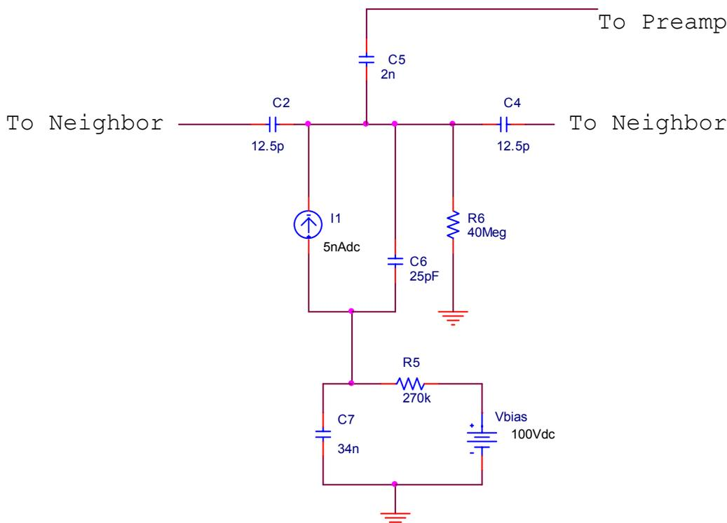
Figure 1. Schematic of the detector model showing one strip plus both interstrip capacitances. There are 23 strips in the model, but only a single bias supply plus filter.
