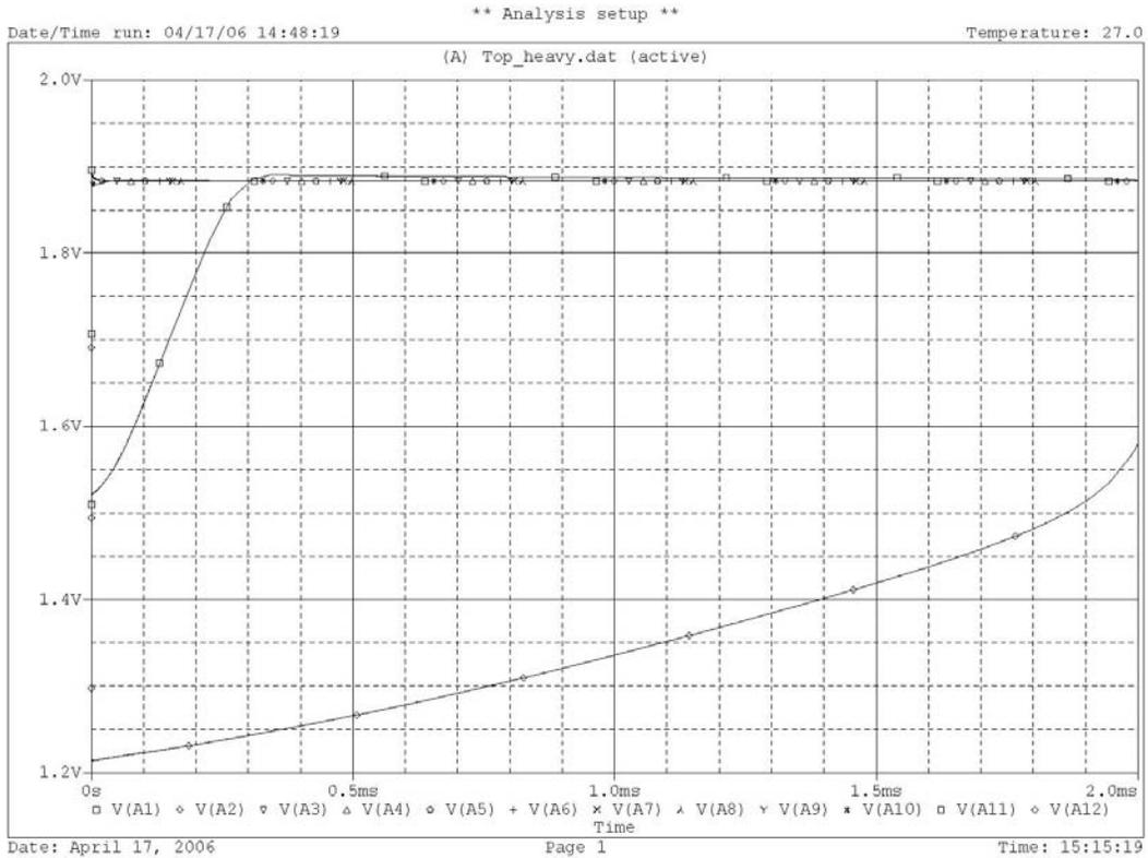
**Figure 5.** The preamp output for an oxygen ion incident on strip 12, shown over a long enough time period to see the decay back to the baseline.
