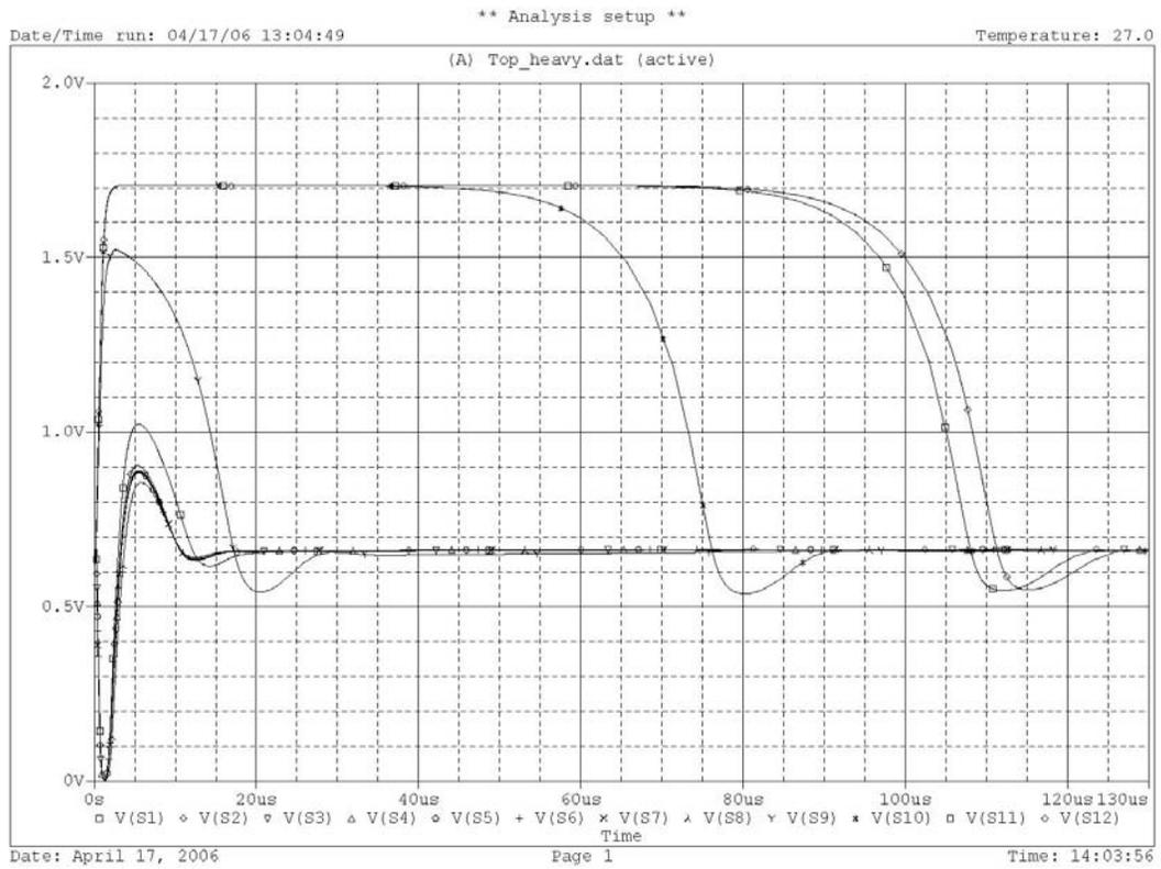
**Figure 7. The shaping amplifier outputs for an iron ion at normal incidence on strip 12.**
