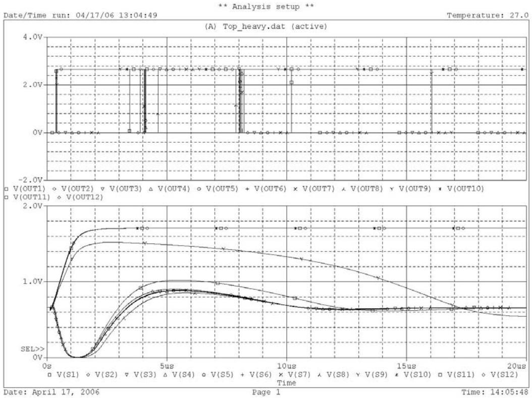
**Figure 8. The shaping amplifier (lower) and comparator (upper) outputs for an iron ion at normal incidence on strip 12.**
