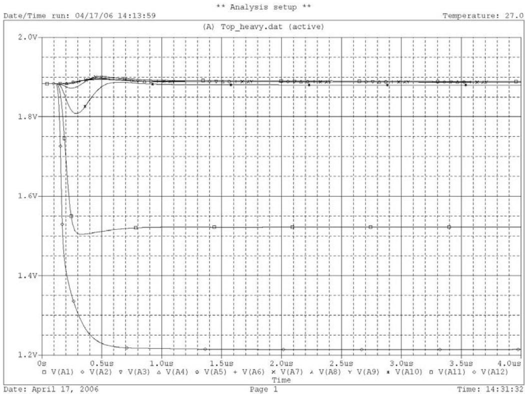
**Figure 2. Preamplifier outputs for the case in which an oxygen ion passes through channel 12.**
