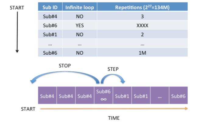
The written configuration is valid until a reset command is sent. This means that, after the configuration phase, the system performs the same sequence each time a START command is sent.
