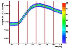
Fit CR-RC pulse shape to determine t<sub>0</sub>
