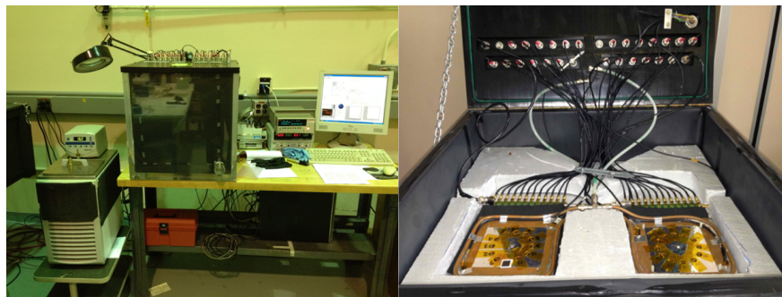
FIG. 3.4.7: On the left, the testing setup is shown and includes a chiller, the light-tight plastic box that contains the LEDs and APDs, an electrometer, and the data acquisition. On the right, the setup inside of the light-tight plastic box is shown that contains a copper cooling plate to maintain the chiller temperature, 10 slots on each side to hold APDs, and the LED in the center of each half.
