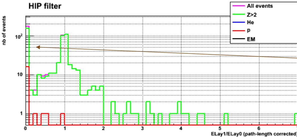
Ratio is -1 when only first layer has a GCR hit
