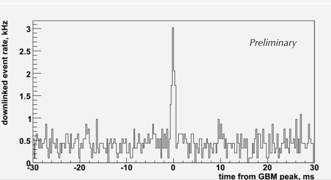
rate and the downlinked event rate. The figure at left shows that, away from the times of TGFs, the mean "trigger request" rate is ~4000 Hz, and the mean downlinked event rate is ~400 Hz, as is typical for LAT. Readily apparent in the figure, however, is an unambiguous excess of events within a millisecond of the TGF peak time.
