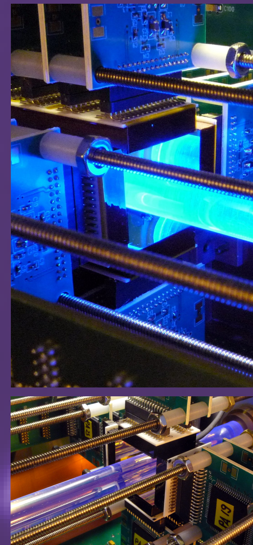
Fig. 2: Incoming X-rays are Compton-scattered (scintillator rod) and subsequently photo-absorbed in a CZT detector.
