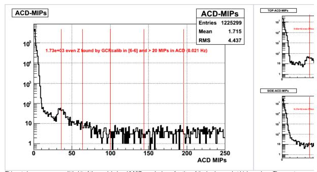
This cut change removes a little bit of the peak below 10 MIPs, and a large fraction of the background at higher values. The spectra on the right panel are for the top tiles (top spectrum) and side tiles (bottom spectrum): the carbon peak has a better peak-to-valley ratio for the top tiles, and it is not visible at all for the tiles on the sides of the ACD.
