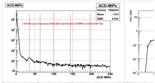
Only the carbon peak is visible. The rate of events above 20 MIPs is 0.06Hz, thus really lower than the ~1Hz of GCRCalib throughput (see right panel). The plot below shows the same spectrum restricted to carbon events. The carbon peak is a bit more pronounced, but still there is less than 1000 hits in all tiles under this peak.
