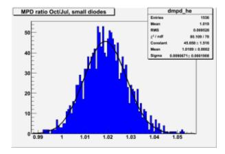
The change in MPD calibration over 3 month is not big ~1.5-2.0% and goes in opposite direction - closer to pre-launch calibration. Anyhow for consistency it is suggested to use the new MPD calibration file.
