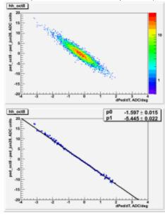
The pedestal drift with respect to currently used calibration is rather significant (between -12 and +18 ADC units), this confirms the need to switch to the recent file.
