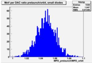
SO, pre-launch MPD coefficients are bigger than the on-orbit ones and now (using pre-launch MPD coefficients) the reconstructed CAL energy is overestimated, especially for small diodes.
