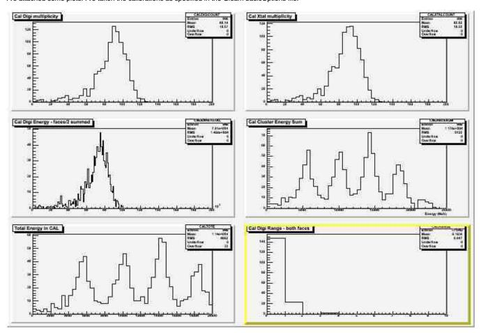
The top two show the hit multiplicity from digi and recon (CalXtalRecData) are consistent. The middle left shows the summed ADC counts for all readouts. Middle right and lower left show energy sums from CalRecon - illustrating the problem. Bottom right shows the range from digi - mostly zero = LEX8. Sure I ooks like a recon problem.
