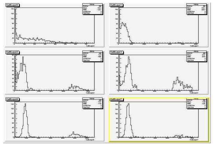
shows layer energies from the Merit tuple - I left off layers 4 & 5; they follow the trend. Note the satellite peaks at 5 GeV.
