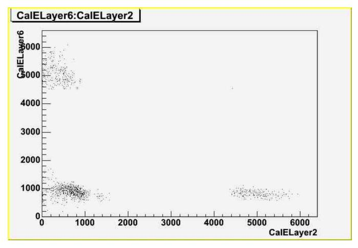
indicates that the satellite peaks are uncorrelated. These plots look like the biggest clue. The layer energies, aside from zero, are all wrong, as seen from the last pre-new-CAL release (v6r2p8) (Merit tuple from systests 10 GeV gammas; GltWord>0):
