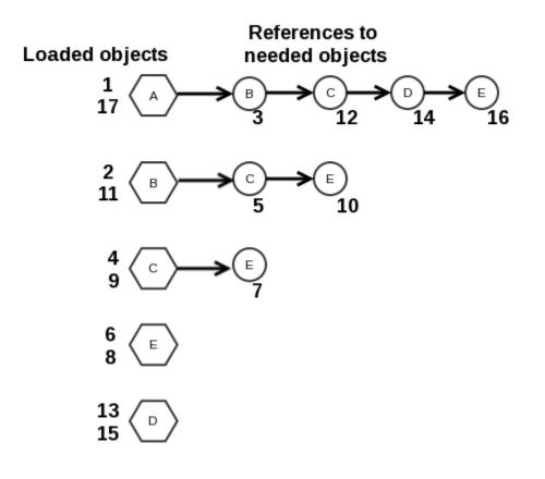
While scanning needed-lists the linker employs a top-down approach; as soon as it sees that an object is needed it loads the object (if needed) then starts scanning the needed-list of the new object. Once the needed-list for a shared object has been completely scanned, the linker then performs the binding for that object.
