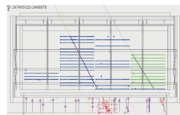
We see that the track on the left, which was originally chosen as the best track, is in fact a ghost, and that the energy of the most energetic CAL cluster in the event (1726 MeV) is actually associated with this ghost track. The cluster associated with the "real" track, on the right, has an energy of 129 MeV. Note that the axes of both of the clusters line up with their corresponding TKR tracks.
