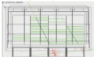
The green horizontal line segments and **X**s show the hit "x" and "y" strips on the silicon detectors in the tracker (TKR), and the blue lines show the found tracks. The "best" track is indicated by the dotted yellow line projecting upward from the head of the track. The red squares at the bottom indicate energy deposited in the calorimeter (CAL); the green box shows the centroid of the deposited energy, and the nearly horizontal green line shows the inferred axis of the shower.
