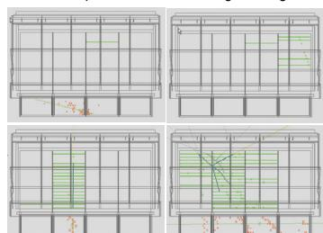
The first has a signal in the CAL, but none in the TKR; the second, vice versa; and the bottom two both have signals in both the CAL and TKR, as well as reconstructed tracks. In principle, there can also be remnant signals in the anti-coincidence detector (ACD), but generally these have a shorter time constant and decay quickly; hence, they are seldom seen.
