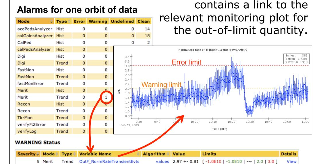
Alarm levels are evaluated for each orbit, on End-Of-Run and trending quantities. We implemented some 20 different alarm algorithms, to check all possible pathological behaviors. Whenever an anomaly is detected, a detailed report is generated and the duty scientists are informed via email.
