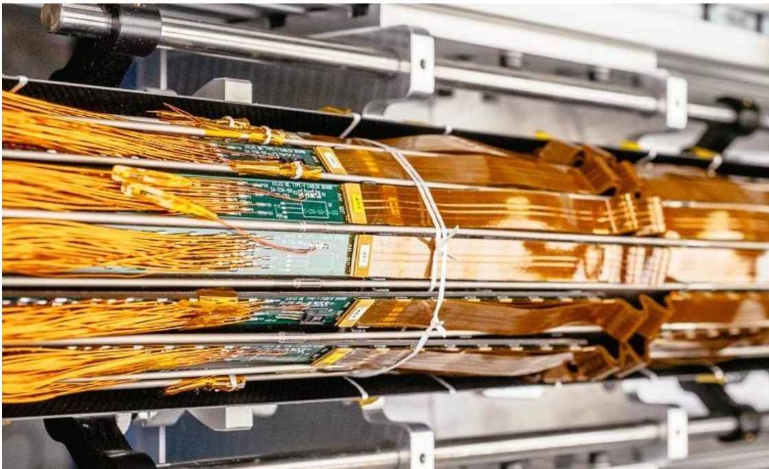
Figure 1-4 PP0 region with fully assembled cable boards and Intermediate Flex connected. The cooling pipe brazing joints at the cable board middle gaps are still visible for the three staves at the front, before NTCs are attached on them.
